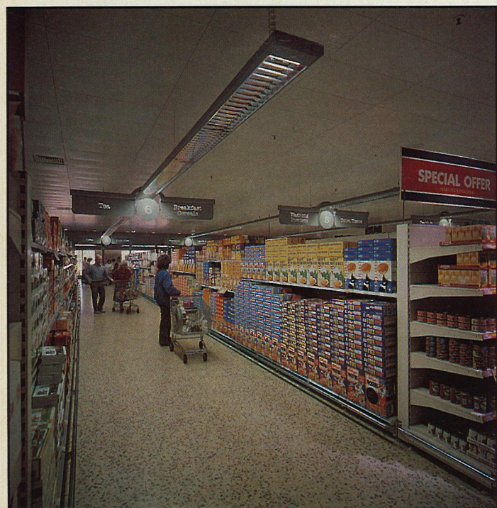
Vertically displayed merchandise is highlighted for more variety and impact with a special system of compact fluorescent fittings with low brightness symmetrical reflectors designed by Thorn Lighting for Tesco.
